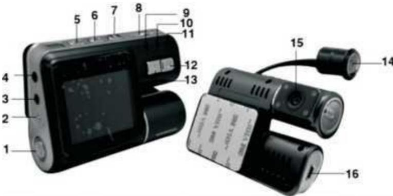
1. Power button (hold down for 3 seconds to turn on/off the equipment)/fill light button
