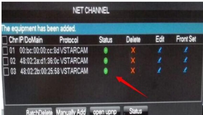
6. The properly connected camera streams the live image to the DVR.
