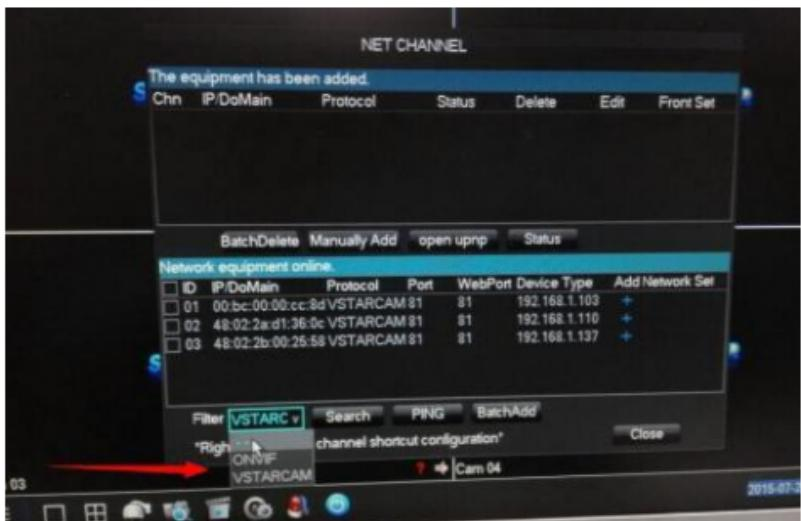
5. Double-click or select the camera detected by the device. A green light shining in the Status window indicates that the camera is properly connected to the DVR. The red one designates a connection error.
