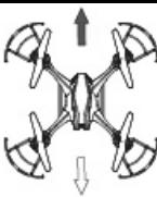
Press the "Forward migration key" if the drone automatically migrates backwards. Press the "Backward migration key" if the drone automatically migrates forwards.
