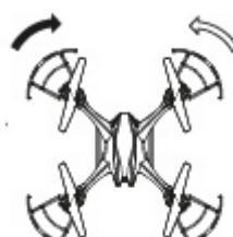
Move the throttle stick left / right to rotate the drone in a given direction.
